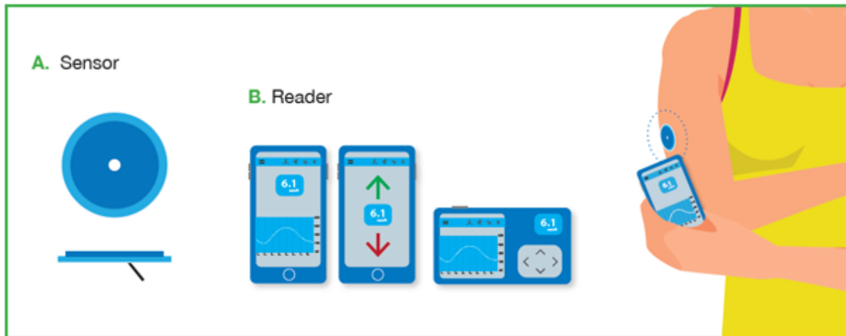
Figure 3.2: Diagram of flash glucose monitoring
