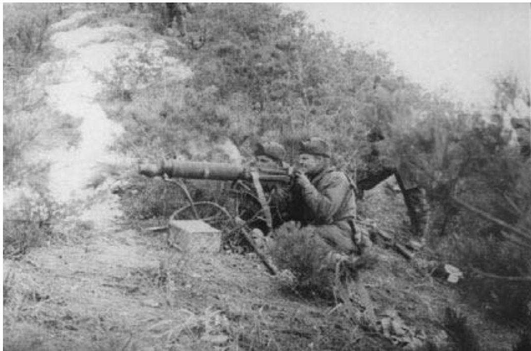
Sergeant Chaperlin, Support Company, 3RAR, engages a Chinese patrol with a Vickers machine gun, Chipyon-Ni, February 1951. The bulbous shape on the muzzle of the gun is a flash suppressor. AWM P1479/07
