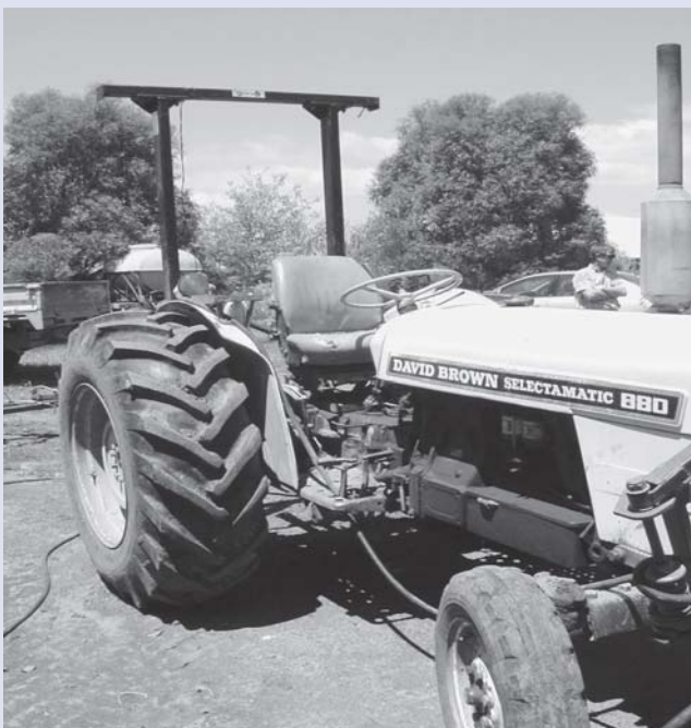
Tractor without access platform
